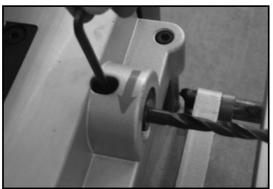
Fix the wood workpiece to the mortising table by tighter the knob (P) and (q). Adjust the table height by the adjusting the handwheel (R)) and fix it at a proper position by locking handle (S).
