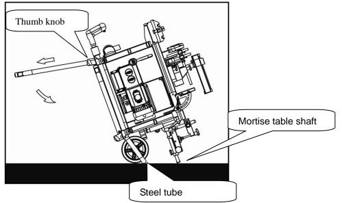
Fix the left and right leg to the machine by the hook.
