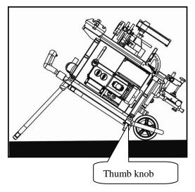
Place the machine on the floor supporting by steel tube and mortise table shaft. Loosen enough the Thumb screws and pull out the left leg, then turn right the left leg.
