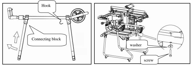
The stand have four circular rubber feet, the machine can be placed steadily by adjusting the four feet.
